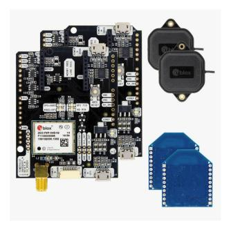
simpleRTK2B - Starter Kit MR has several different configurations to provide you with flexibility:
