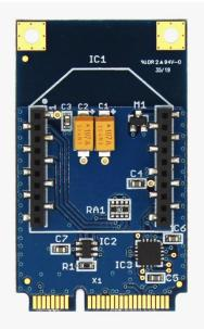
mPCIe Carrier Board for XBee Plugins SKU is: AS-ADP-XBEE-TO-MPCIE-00
